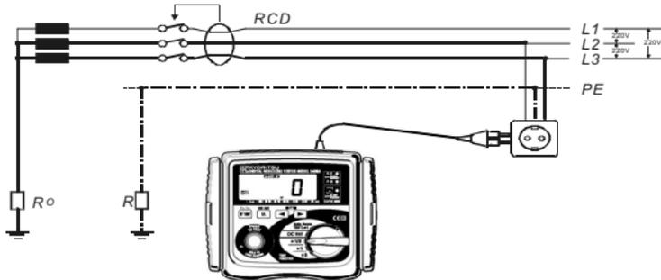
Connecting the model 5406A to this system, all three wiring check LEDs should be lit.
