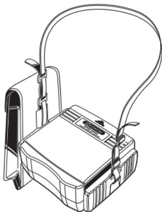
Pass the strap through the buckle, adjust the strap for length and secure.
